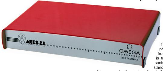
The Ares 21 is an intelligent input/ output interface with an onboard buffer memory. Timing data is recorded for each input port and identified with a unique alphanumeric code. Data from the Ares interface is transmitted to the associated computer via a standard serial line. All
