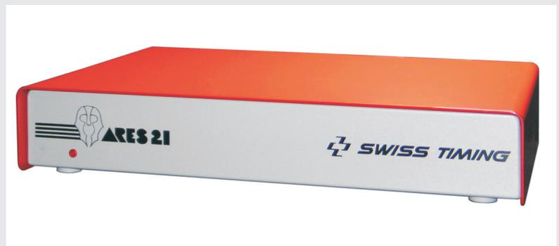
the main results printer or to a full matrix scoreboard. Protocol information can be provided to designers of external results systems to enable start lists to be downloaded from the results system into the Ares 21 database and for timing data to be uploaded from Ares into the results system.
